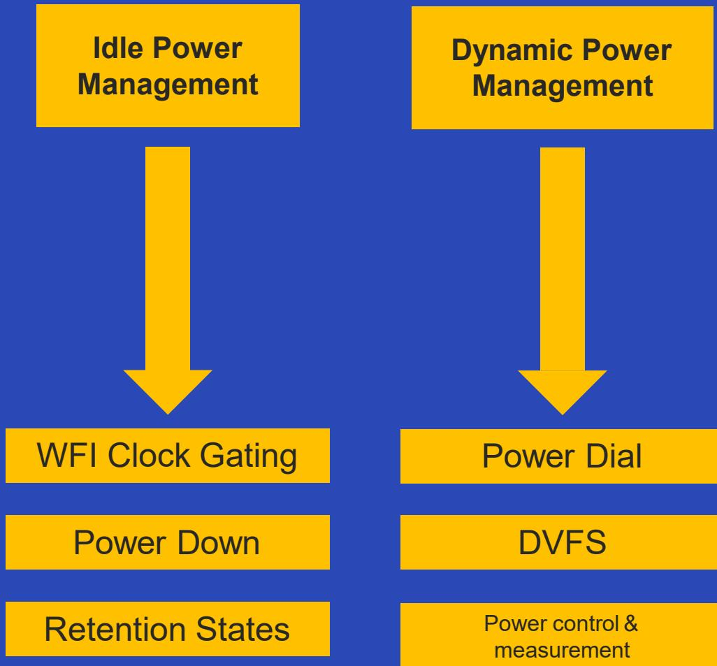
SiFive Power Dial: Digital Throttle to Reduce Power Performance vs. Power
