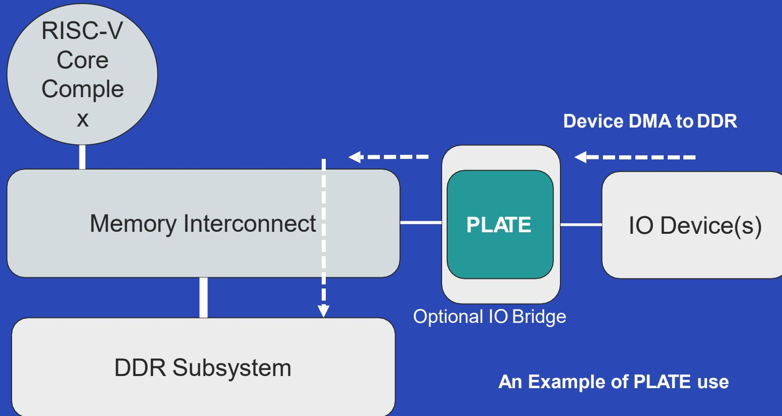
SiFive-specific IP enables fast yet protected DMA
