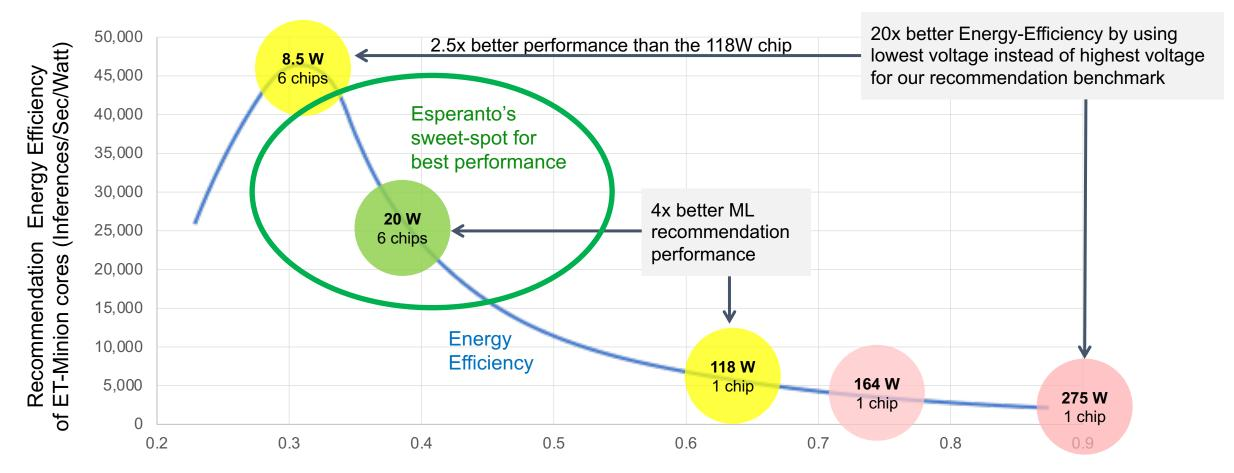
Operating voltage for the 1K ET-Minion RISC-V/Tensor cores
