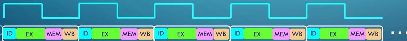
Single-Stage architecture returns to the original program on the next clock cycle after branch or interrupt completes, eliminating the need to discard the loaded program or reload the program as in pipelined processing, thus preventing operational delays. This improved operation results in highly efficient operation.
