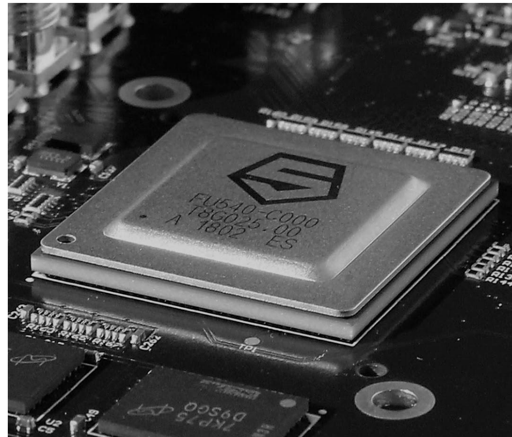
Freedom U540, FCBGA, manufactured in TSMC 28nm
