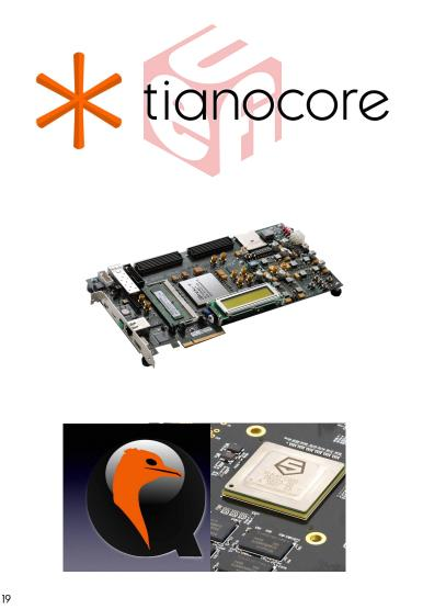
Last year, HPE engineers have made Tianocore successfully boot on SiFive Freedom U500 VC707 FPGA Dev Kit(with USB3.0 and PCIe 3.0 support).
