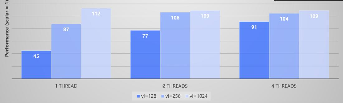
\* Measurements are under development. The scalar code is highly optimized (unrolled loop). L2 cache status assumes a cold start.
