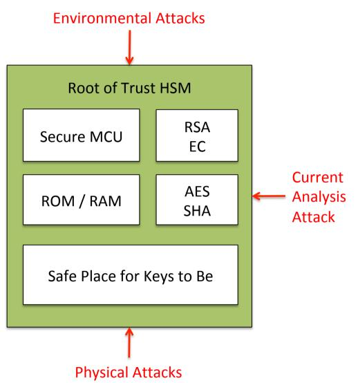
Because HSM is simple, it can incorporate original ideas that are not hacked at the architecture, microarchitecture, and logic implementation levels.
